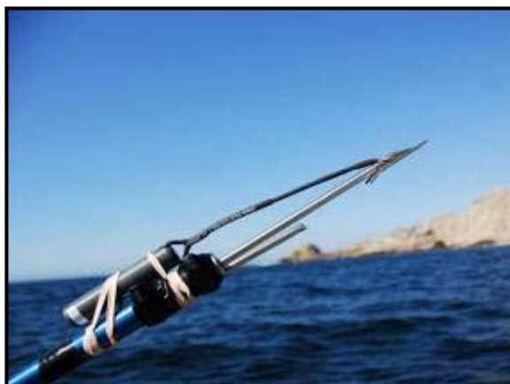
Figure 9. Pop-up satellite archival tag attached to a titanium barb on a pole spear. Note the metal tube beneath the spear shaft that would collect biopsy samples. (Courtesy of Sal Jorgensen.)
