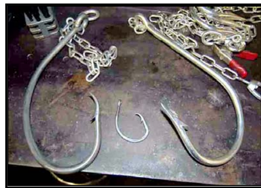
Figure 8. Circle hooks (left and center) compared to J-hook (right). The hook shown on the left is proposed to be used, which is 13 inches long by 7 inches wide, with a 5-inch gap between the point and the shank (Courtesy of Michael Domeier.)
