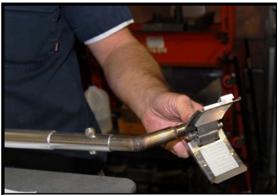
Figure 22. Spring-loaded attachment device for real-time satellite tags. (Courtesy of Michael Domeier.)
