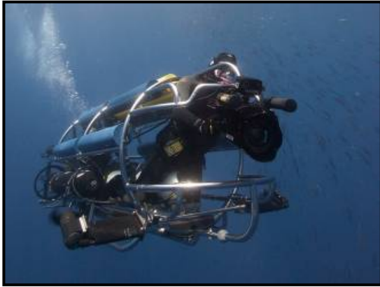
Figure 15. Underwater mobile shark cage. (Courtesy of James Moskito, Great White Adventures, Inc.)
