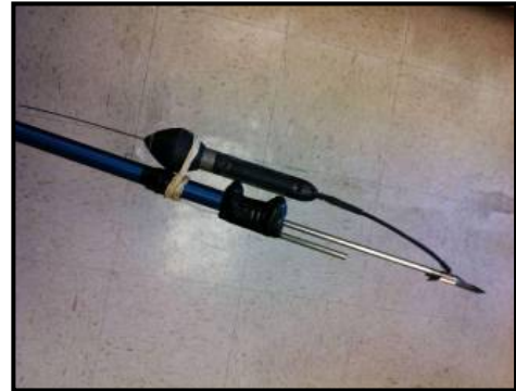
Figure 12. Acoustic monitoring tag attached to a titanium barb on a pole spear. Note the metal tube beneath the spear shaft that is used to collect biopsy samples. (Courtesy of Sal Jorgensen.)
