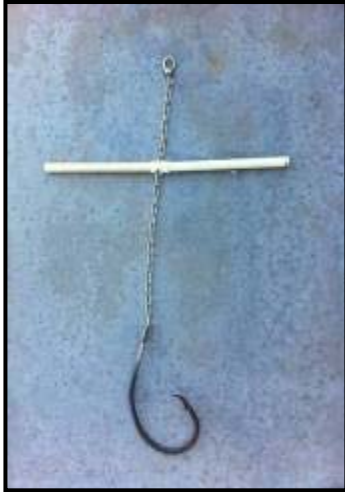
Figure 24. A blocker-type of device to better assure that white sharks are hooked only in the mouth. (Courtesy of Michael Domeier.)
